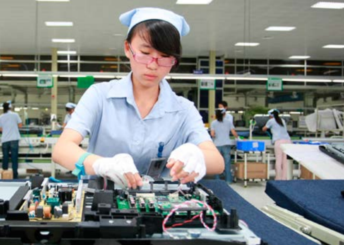
LCD television screens are assembled in Chengdu in Western China
